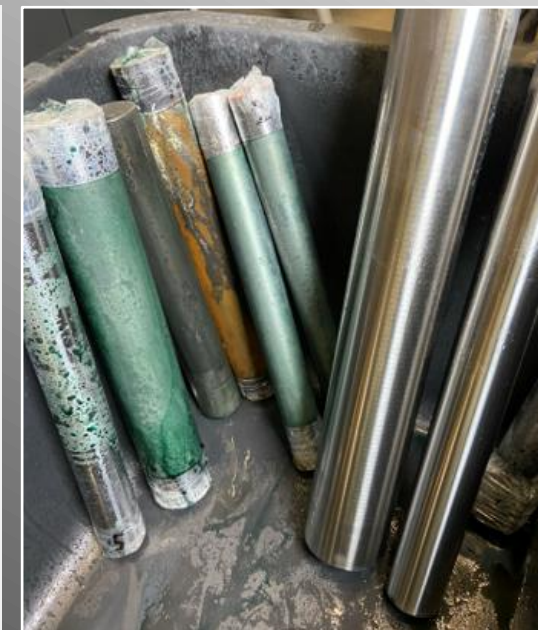
Commercial Cr 6+ coatings vs. TripleHard® after 5 days of mine water spraying
