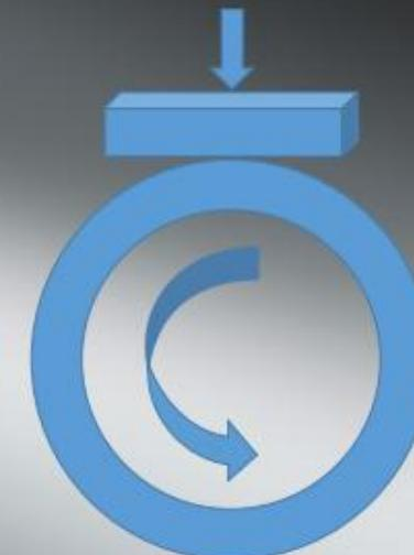
BOR is a harsh test that is commonly used method in the industry to investigate resistance of materials and coatings, like in linkage pins. In this test, TripleHard® was compared to hexavalentchromium, which did not resist until the end of the test. That is indicated by the spike in the friction graph. TripleHard® resisted until the end of the test with the maximum load.
