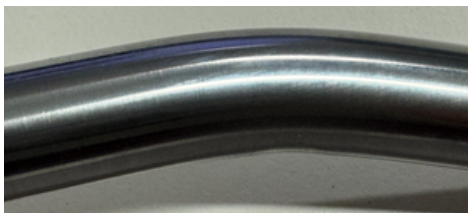
Bend test - No detachment, ensuring strong adhesion
