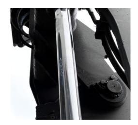
TripleHard® surface consists of a dual-layer system combining nickel and trivalent chromium. The nickel
